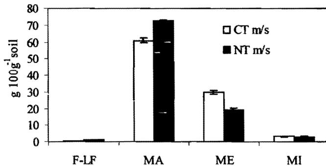
Figure 4-1 : Aggregate size distribution in conventional-tillage (CT m/s) and no-tillage (NT m/s) soils, 0-5 cm layer. (Andranomanelatra, Madagascar). F-LF = Free-light fraction; MA, ME and MI = macro-(200-2000  $\mu\text{m}$ ), meso-(20-200  $\mu\text{m}$ ) and micro-(0-20  $\mu\text{m}$ ) aggregates, respectively.
